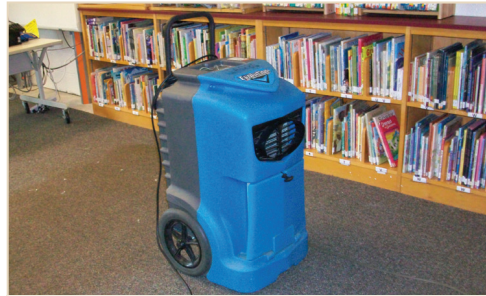
PHOTO 3 Portable dehumidifier installed in classroom.
