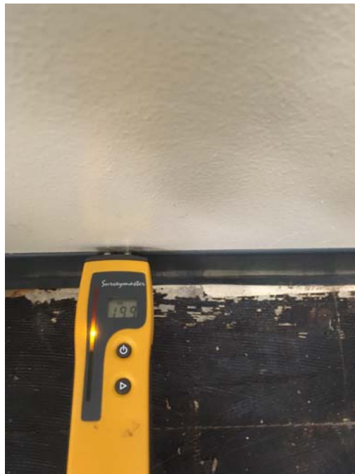
Photo 4 – Room 102 Elevated moisture content was detected on the wallboard below the section of mold growth.
