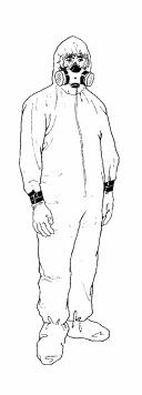
**Respirator:** The DEQ suggests you purchase a dual cartridge respirator equipped with two HEPA (high efficiency particulate air) filters for use on this project. The HEPA cartridges are color-coded purple or magenta. Ask your vendor for a fit test to make sure that your respirator fits properly.
