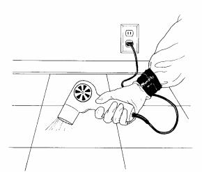
5. Tile Repair: For single tile removal or small repair areas you may be able to use a heat gun (not a hair dryer), dry ice, or solvent.
