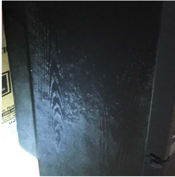
Photo 29 – Small Teacher's Storage Room Mold growth was observed on the TV cabinet.
